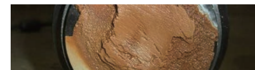
Debris Buildup Around the Detection Section
